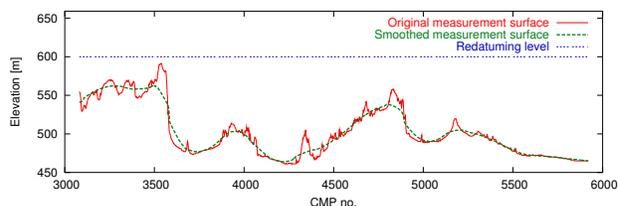
Fig. 1: Comparison between original and smoothed measurement surface. The horizontal redatuming level at  $z = 600$  m is also displayed.
