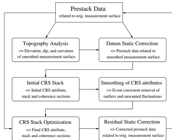
Fig. 2: Cascaded processing scheme to handle topography in CRS stack and residual static correction.
