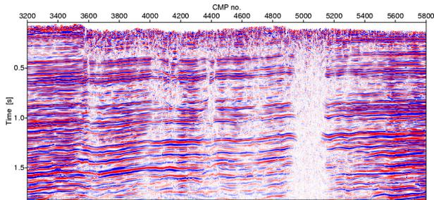
Fig. 5: CRS stack section after residual static correction and redatuming, related to a fictitious horizontal measurement surface at  $z = 600$  m. Note the reduced acquisition footprint around CMP no. 3600 compared to Figure 4.
