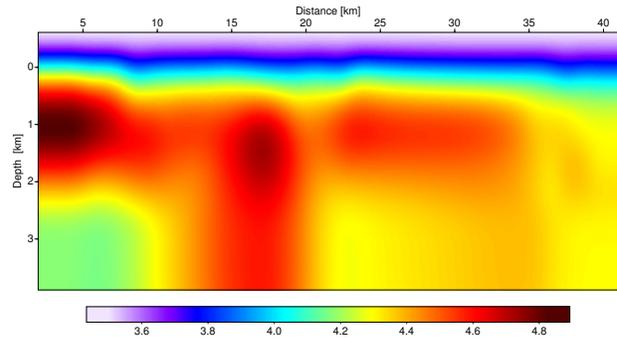
Fig. 6: Macrovelocity model [km/s] obtained by CRS-attribute-based tomographic inversion.
