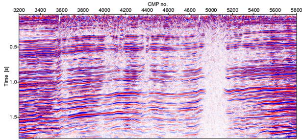
Fig. 4: CRS stack section after residual static correction
