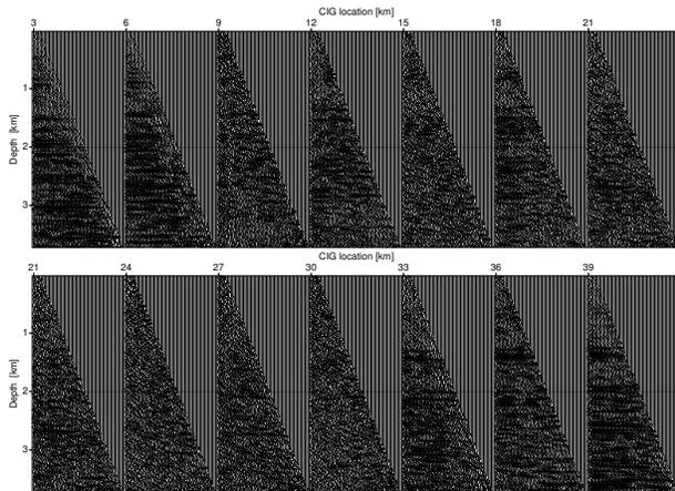
Fig. 8: Some common-image gathers extracted from the prestack depth migration result before stacking over all offsets.
