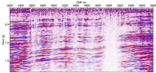
Fig. 3: CRS stack section
