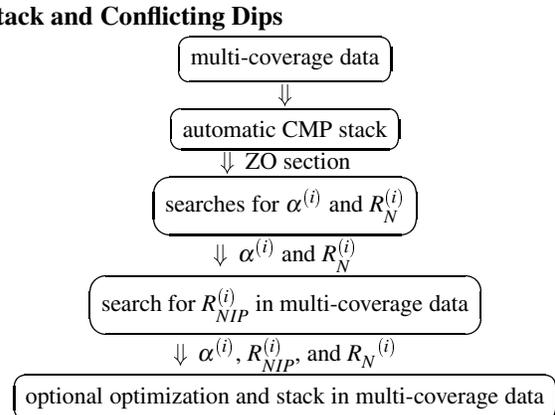
Fig. 5: Simplified flowchart of the adapted search strategy. The index  $i$  denotes the different events detected for one and the same ZO sample.
