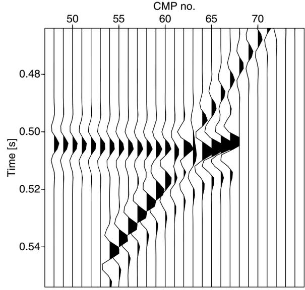
Fig. 2: Detail of the modeled ZO section of the synthetic data set used as input for the result shown in Figure 1. The interference of the intersecting bow-tie segments is clearly visible.
