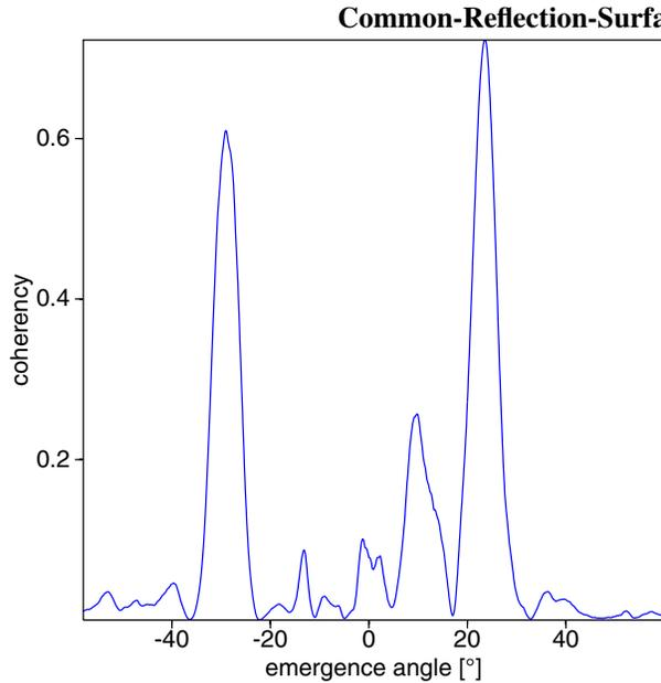
Fig. 4: Coherency measure plotted versus the tested angles of emergence of the normal ray. Distinct local maxima can be observed, although conflicting dips have not been considered in the preceding step.
