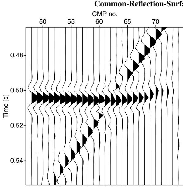
Fig. 1: Detail of a simulated ZO section for a synthetic data set. Conflicting dips are not considered in this application of the CRS stack, therefore the steeper bow-tie segment is broken instead of interfering with the flat bow-tie segment.
