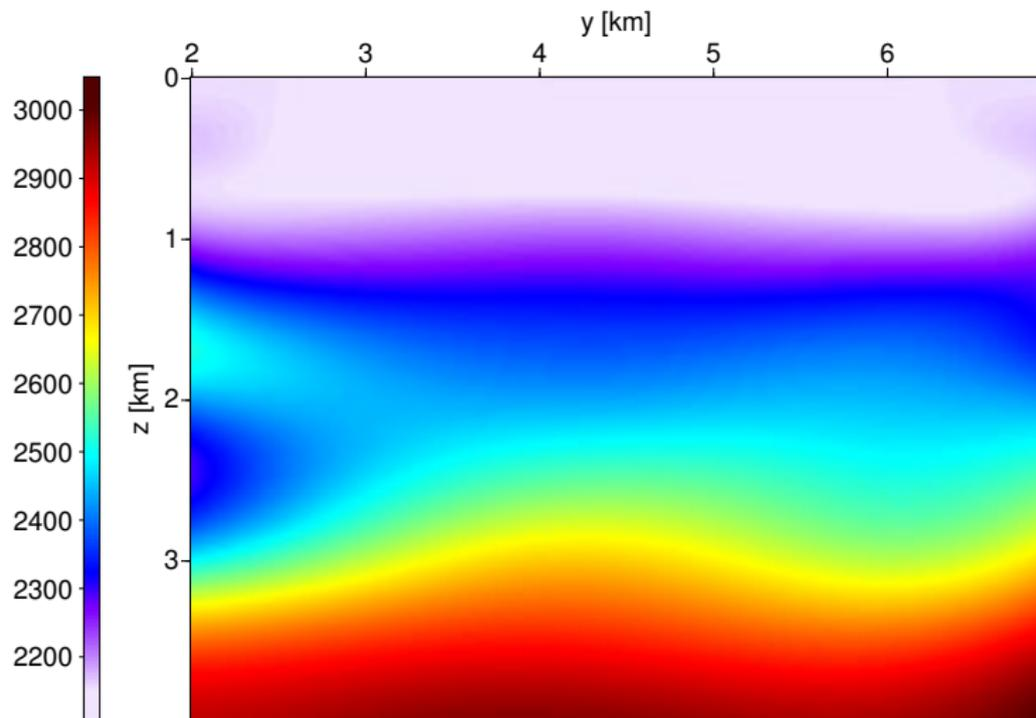
reconstructed velocity [m/s] model at  $x = 5000$  m
