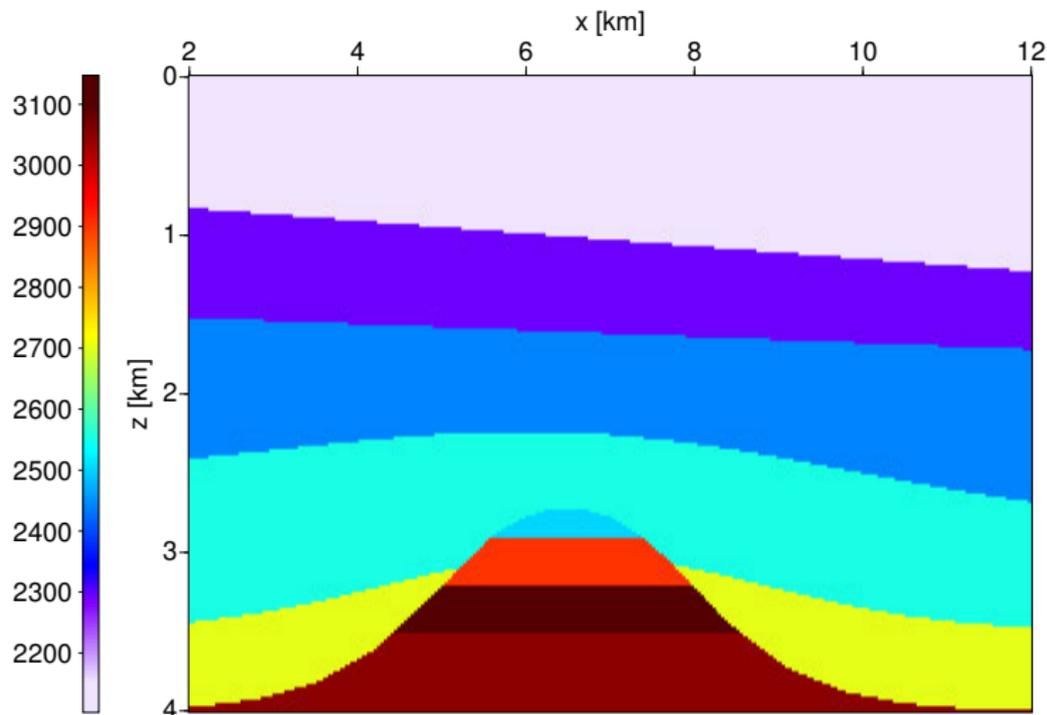
interval velocity [m/s] model at  $y = 5000$  m
