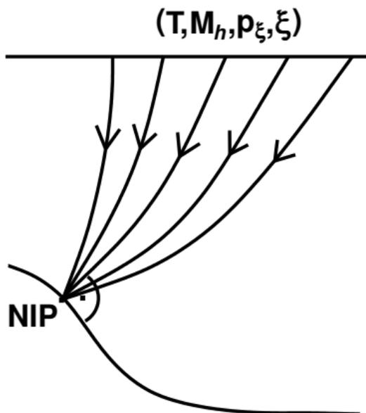
In consistent velocity models, NIP waves focus at zero traveltime.
