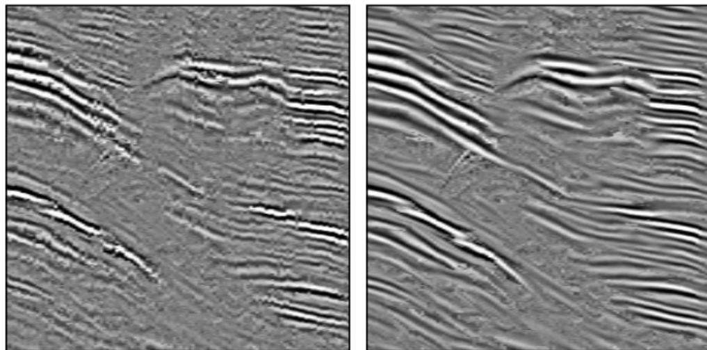
Stack with original vs. stack with smoothed parameters
