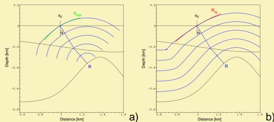
Figure 1: Two hypothetical experiments: a) *NIP* wave for a point source at R, b) *normal* wave for an exploding reflector. The central ray is shown as a dashed line.
