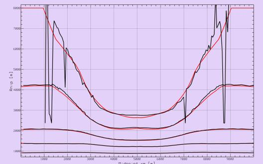
Figure 8: Model-derived (red) and data-derived (black) radii of curvature of the *NIP* waves for all layers.
