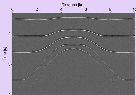
Figure 6: Stacked section as final result of the optimized CRS stack.
