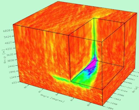
Figure 4: Coherency depending on the wavefield attributes for the depth point R depicted in Figure 3. The excavated block exposes the global maximum.
