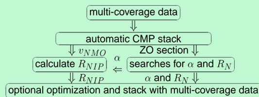
Figure 5: Simplified flowchart of the pragmatic approach to determine the wavefield attributes.
