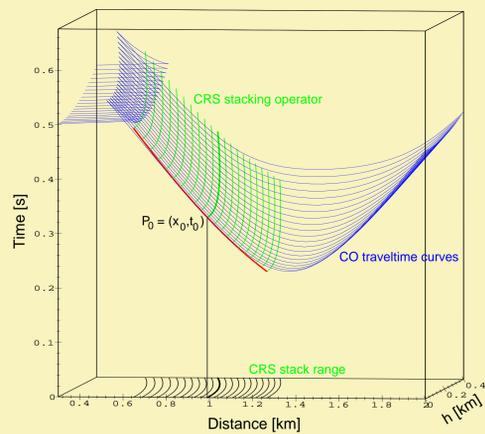
Figure 2: Forward calculated traveltimes surface (blue) compared to the CRS stacking operator (green) according to the true (model-derived) attributes. In the zero-offset plane the operator is depicted in red. The CRS stack range corresponds to a paraxial vicinity of the central ray.
