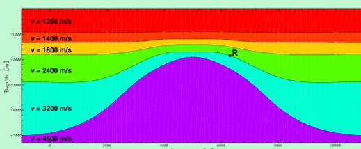
Figure 3: Model with homogeneous layers and dome-like interfaces. We simulated all primary events with a Ricker wavelet (30 Hz peak frequency) and a signal-to-noise ratio of 4.
